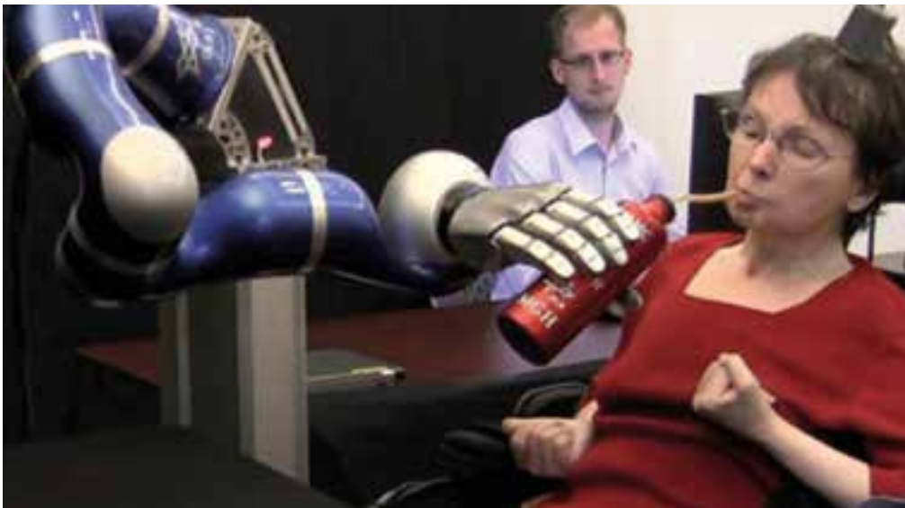
Left: A clinical trial of the cortical implant 'BrainGate' demonstrates how a person with paralysis is able to control a robotic arm using just their thoughts. © Brown University.
