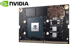
Jetson Nano delivers 472 GFLOPs and can run AI models at just 5 to 10 watts.
