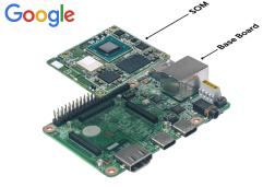
The Edge TPU is an ASIC chip designed to run TensorFlow Lite ML models at the edge. The dev kit includes a system on module (SOM) that combines Google's Edge TPU, a NXP CPU, Wi-Fi, and microchip's secure element in a compact form factor.
